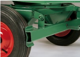
How to brake: Lift drawbar - beam presses on wheels and brakes hand truck Order no.: G1 0612 000
